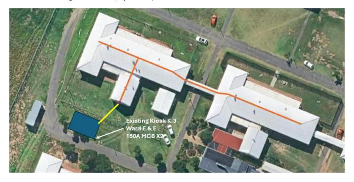
Existing kiosk K.3 has 2x150A circuit breakers servicing ward E and ward F. The cables shall be rerouted into container power control distribution board and the kiosk dismantled. The feed cable shall feed the changeover and the inverter input via dedicated circuit breakers.
