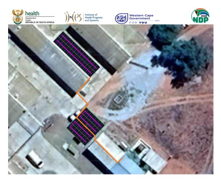
The output feed shall be run out of the building towards the generator into an existing covered trench and pulled into the essential power distribution board where feed-in shall occur into the reticulation.
